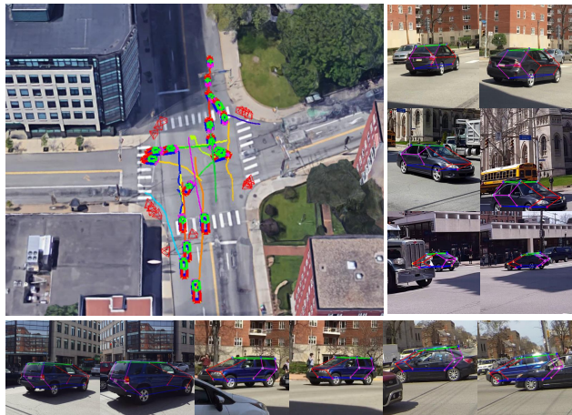
Figure 1: Reconstruction of vehicles crossing a busy intersection, making turns, going straight and changing lanes. A subset of vehicle skeletons (3D detector locations) and their 3D trajectories are augmented within the Google Earth view of the intersection. The reconstructions are reprojected into multiple views of two cars (a sedan and an SUV) demonstrating good performance under partial occlusions.
