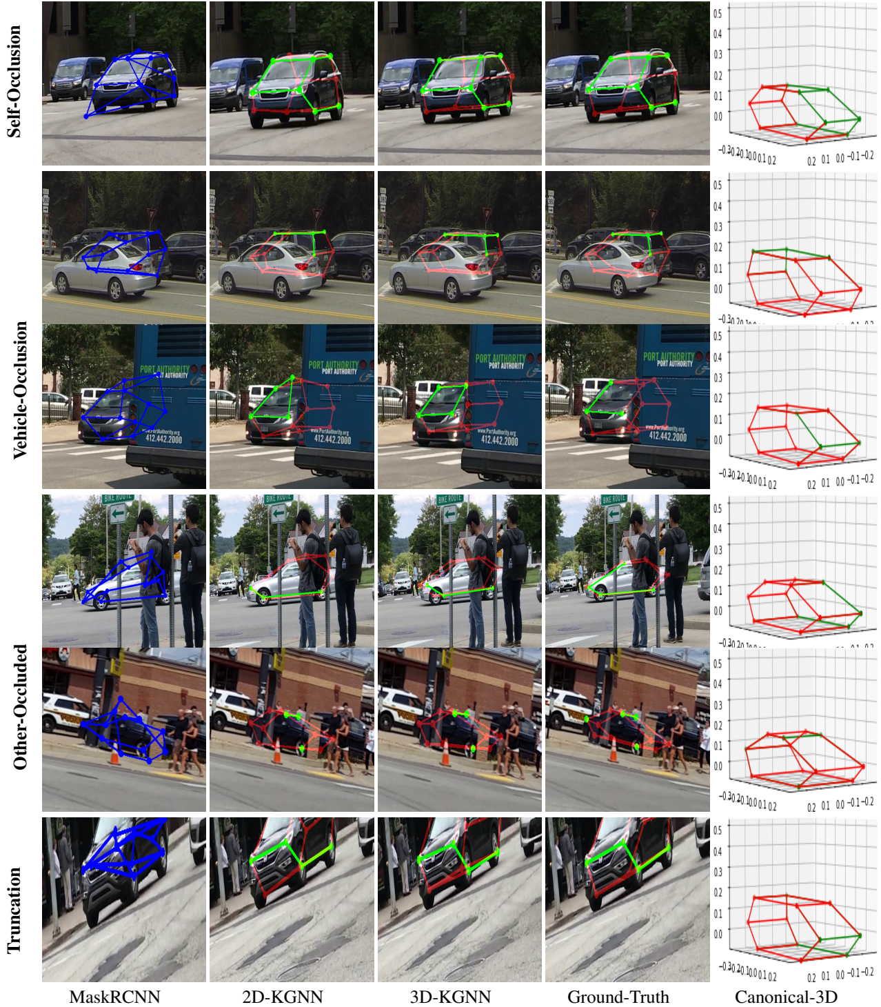
Figure 11: Qualitative evaluation of the 2D/3D keypoint localization for different occlusion categories of cars from the CarFusion dataset. The initial detector was trained using the MaskRCNN on the visible 2D keypoints. We use our self-supervised 2D-KGNN and 3D-GNN to localize keypoints from a single view. 2D reprojections of the 3D keypoints are shown in third column. The second and third columns show clear improvement in the localization of the occluded keypoints with respect to the baseline MaskRCNN. The canonical 3D views computed using 3D-KGNN are shown in the last column. The ground truth is obtained by applying trifocal tensor on the human labeled visible points to estimate the invisible points. Green represents visible edges and red represents occluded edges.
