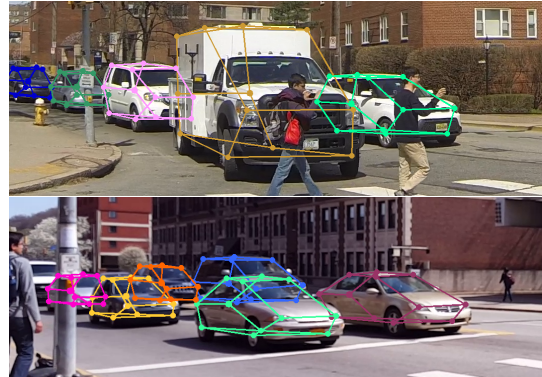
Figure 1: Accurate 2D keypoint localization under severe occlusion in our CarFusion dataset. Different colors depicts different objects in the scene.
