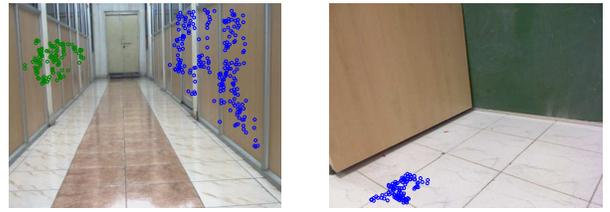
Figure 3: Planar patches obtained after the distance based refinement step for corridor and corner dataset. In comparison to Fig 2, the images show that our distance based refinement step is able to cut the detected scene planes (that spanned two or more real world planes) into smaller planar patches (that span only a single scene plane).
