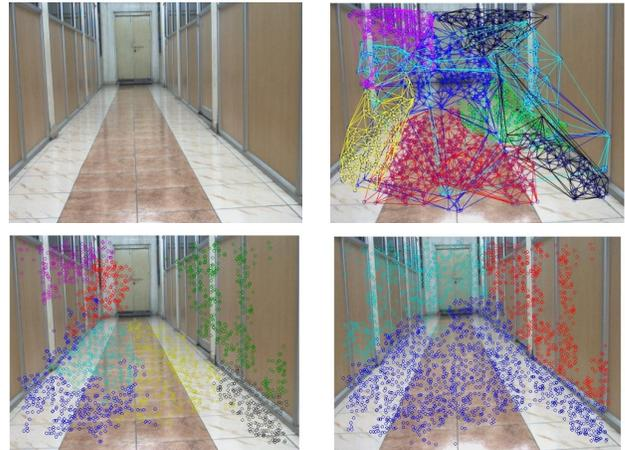
**Figure 1: Multiple Plane detection from images. Top Left Initial Image to be segmented. Top Right Initial planar patches detected from ORK. Bottom Left Refined patches after distance based segmentation of planes Bottom Right Multiple planes detected corresponding to scene planes after optimal MRF labelling.**
