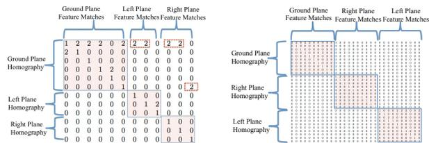
Figure 4: The minimum and second minimum after applying the homography of one plane to feature matches of the other.
