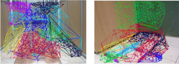
Figure 2: Scene planes detected for corridor, corner dataset respectively (from left). Connected meshes with the same color indicate matches that are grouped together as belonging to one plane by [2].
